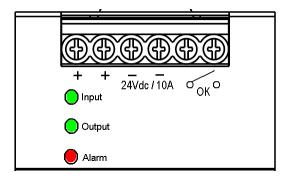
Three user-friendly LEDs for status and diagnostics Shows status of input power, output power and alarm condition Valuable troubleshooting aid to reduce system downtime
