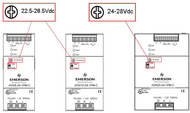
**Single / Parallel switch** - The outputs of two or more of ADN-C series power supplies can be connected in parallel to increase the total current capability. When operate the ADN-C power supplies in parallel, the Single / Parallel switch on each of the ADN-C power supply should be placed in the parallel position. Units will not be damaged by parallel operation (regardless of switch position setting)
